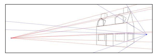
Complete the picture of the house. You will need to draw perspective guide lines to help you create an accurate drawing of the house. 使用视角线精确地画出下列房屋图。
