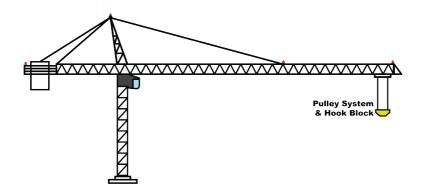
There are many real wold applications for pulley systems. Elevators, exercise machines, and toys are just a few examples of how pulleys get used. Tower cranes also use pulley systems which are attached to a hook block to lift heavy loads. By using custom pulley systems the Mechanical Advantage ( $M_A$ ) of a tower crane can allow crane operators to lift heavy loads that typically weigh thousands of kilograms.
