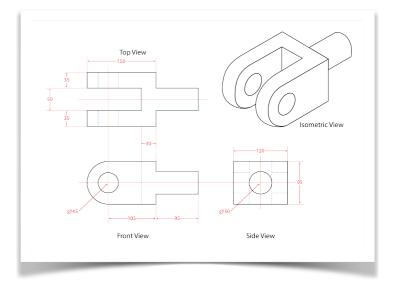
Orthographic drawing show schematic details of an object. Typically Orthographic Drawing are done in CAD software (Computer Aided Design Software). Every machined product was first design as an Orthographic drawing in a CAD program before it was manufactured. Every toy, car part, even the pens you use in class were all designed in a CAD program before a machine made each product you use everyday.
