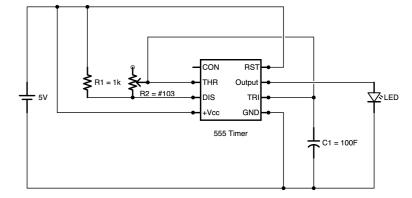
This simple 555 timer circuit can be used to produce a square wave in which the **T1 (High Time)** and the **T2 (Low Time)** can be calculated. This method of determining specific values ahead of time is used by electrical engineers to control the rate that an LED will blink. The final output obtained from **Pin 3 (Output)** is by the graph "**555 Timer Circuit Duty Cycles**":
